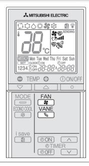
Press 50 to select fan speed. Each press changes fan speed in the following order:
