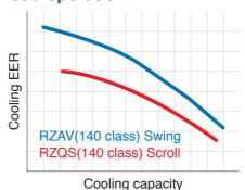
Swing compressor can operate lower minimum capacity compared to scroll compressor.
