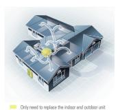
The Daikin Premium Inverter can be retrofitted onto an existing R22 system by simply replacing both the indoor and outdoor units whilst retaining the field piping intact\*.
