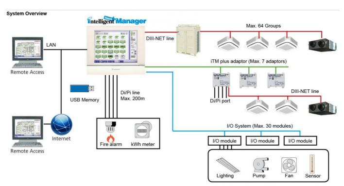
Through the intelligent Touch Manager (ITM), you can now control all Daikin VRV, Sky and RA products simply and conveniently. Each ITM is equipped with a single DIII Net port that enables control over 64 indoor unit groups and up to 10 outdoor systems.
