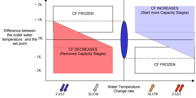
In order to anticipate, the reference point is recalculated each time the difference between air temperature and set point reach a minimum or a maximum.
