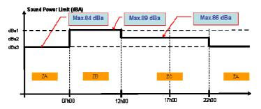
The Climactic<sup>™</sup>50 can manage 3 different strategies for the fan and compressors, defined by the setting (3611): NOT USED, QUIET, QUIET++. This set point controls the fan capacity (%) and the compressors in case of condensing pressure too high.
