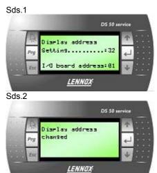
Access the configuration mode by pressing the buttons  $\uparrow \downarrow \leftarrow \downarrow$ , for at least 5 seconds until the Sds.1 screen appears: Press button  $\leftarrow \downarrow$  to position the cursor over the 'Setting' line With the  $\uparrow$  or  $\downarrow$  button, set the address of the display to 00 (instead of the standard value of 32) and confirm with button  $\leftarrow$
