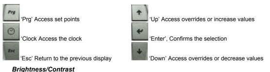
The display has a set contrast, but this can be adjusted manually. For manual adjustment of the contrast, press the 'Prg' and 'Clock buttons simultaneously and press buttons  $\uparrow$  or  $\downarrow$ , to increase or reduce the contrast.
