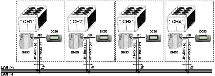
The intercard bus (pLan) is connected to Climatic<sup>™</sup>50 on the J11 connector of board BM50.
