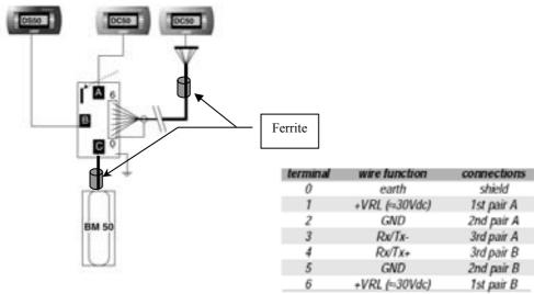
BM50 on connector 'C', DC50 on connector 'A' or 'C', DS50 on connector 'B'.
