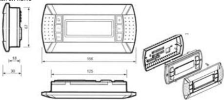
Display DC50 or DM50 is connected to the Climatic<sup>™</sup> with the DT50 screw connector.
