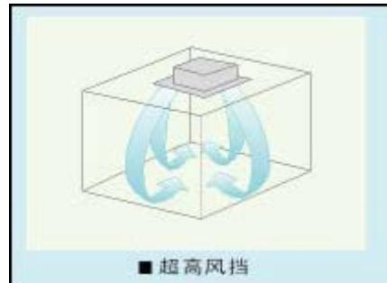
1.15) Reserve spaces for air side-outlet, it is available to connect duct pipe hence Air supplying from the four sides to nearby small room.
