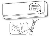
Check that the reception buzzer sound "peep" is emitted from the indoor unit.
