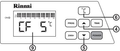
If the set temperature is set to CF 5 °C then the constant frost protection program will be activated. This is useful during winter in alpine areas where the ambient temperature is likely to fall below 5° C.
