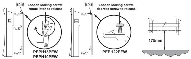
2. For models **PEPH15PEW** & **PEPH10PEW**, loosen the locking screw and rotate the locking latch on the taller leg of the mounting bracket and detach the mounting bracket from the back of the panel heater.
