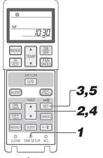
Press the TIME SET UP switch.
