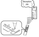
Check that the reception buzzer sound "pip" is emitted from the indoor unit.
