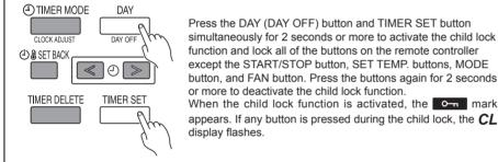
Press the DAY (DAY OFF) button and TIMER SET button simultaneously for 2 seconds or more to activate the child lock function and lock all of the buttons on the remote controller except the START/STOP button, SET TEMP. buttons, MODE button, and FAN button. Press the buttons again for 2 seconds or more to deactivate the child lock function. When the child lock function is activated, the om mark
